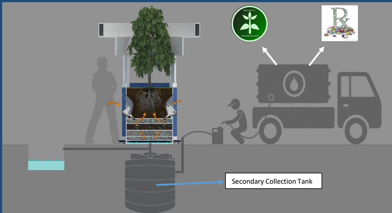
Fig. D) Flow of Urine: Collection of urine for use in Agriculture and Pharmaceutical Drug Manufacture
