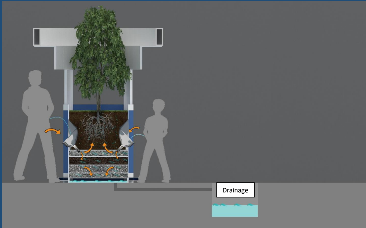
Fig. C) Flow of Urine: Disposal of urine to sewage system
